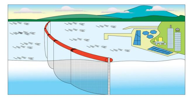
Image by Skimoil. A turbidity curtain is a protective barrier created within the dredging area to contain any sediment (sand and mud) that may be suspended in the water during dredging operations. This barrier is made of an orange floating boom that sits atop the water surface and a suspended curtain that hangs down into the water.
